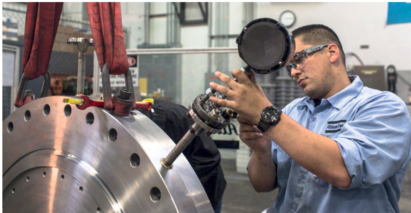
A turboexpander is assembled for a hydrostatic test.
