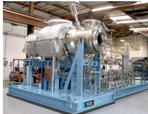
A turboexpander for cryogenic hydrocarbon separation.
