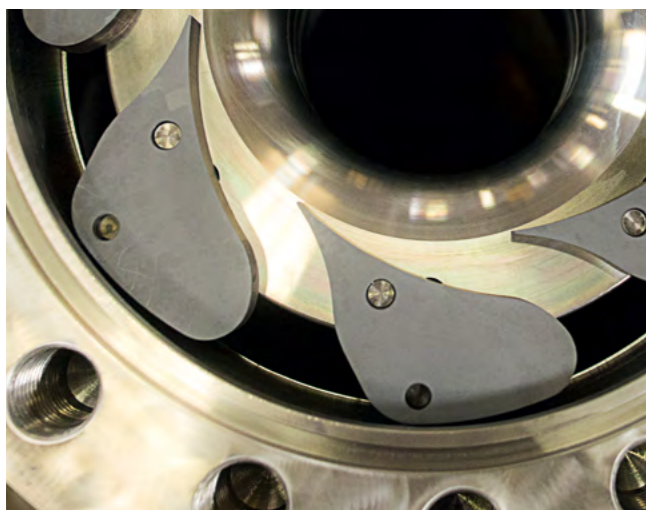
Variable inlet guide vanes enable optimum performance across a full range of process conditions.
